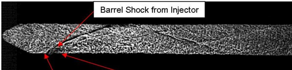
Barrel Shock from Injector
