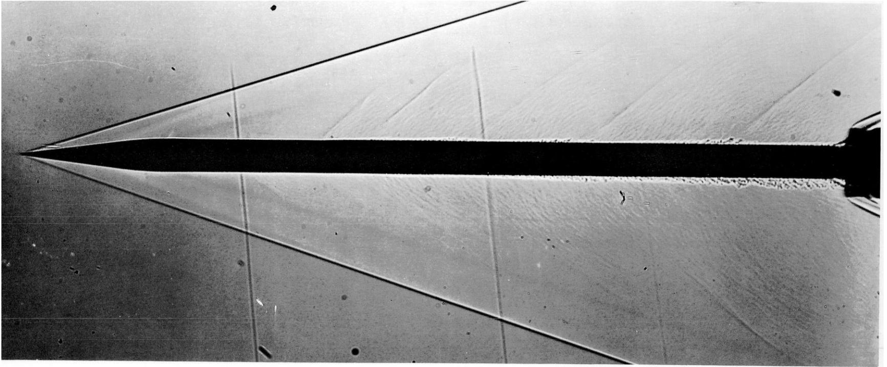
Shadowgraph of conical-nosed cylinder model in free flight;  $M_\infty = 3.5$ ;  $U_e/\nu = 2.1 \times 10^6$  per inch;  $H = 150 \mu\text{in.}$ ; wind tunnel "air-off"; conical light field.
